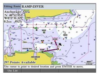
4. Use the **ROCKER** to drag the map pointer to the location where you want to move the route point, and then press **ENTER** to move the route point.
